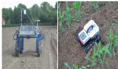
Figure 18 (Left) Portal robot (Madsen and (Right) Sub canopy robot ISAAC2 built by a student team from Hohenheim University
