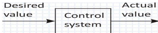
Fig. 8 Open Loop System
