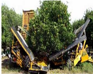
Fig. 25 Citrus harvester – Tree shaker Source: University of Florida, Citrus Mechanical Harvester website
