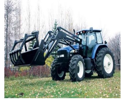
Fig. 28 Modern Tractor with hydraulic front-end loader Source: http://static.wixstatic.com/media/7c998a_ef6be35f071331a566065086a30830d9.jpg_1024
