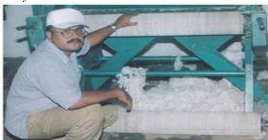
Figure-9: Green Design of Gin Rollers of Double Roller Cotton Ginning Machine
