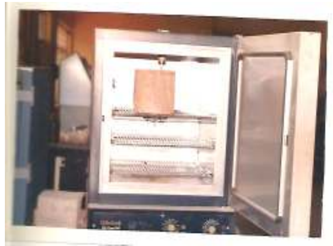
Plate 1: Sample of specimen inside the oven
