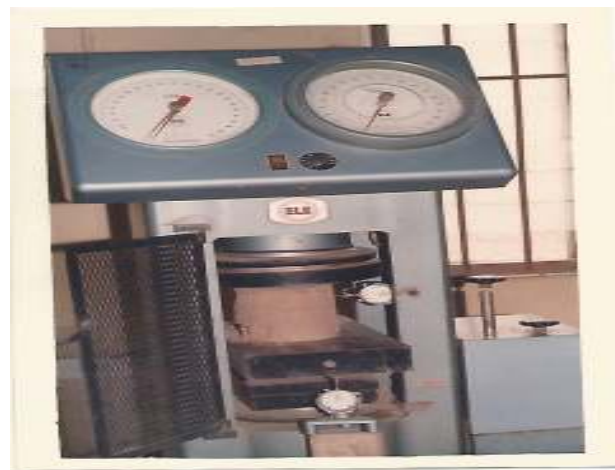
Plate 2: Compression machine armed with dial gauges
