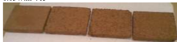
Figure 3: Images of Illite Clay in different volume fraction of granular cork
